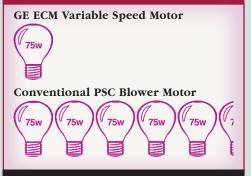
On continuous fan, the GE ECM variable speed motor will use approximately 75 watts of power compared to a conventional PSC blower motor that can use over 400 watts.
